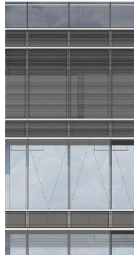
CURTAIN WALL ELEVATION
